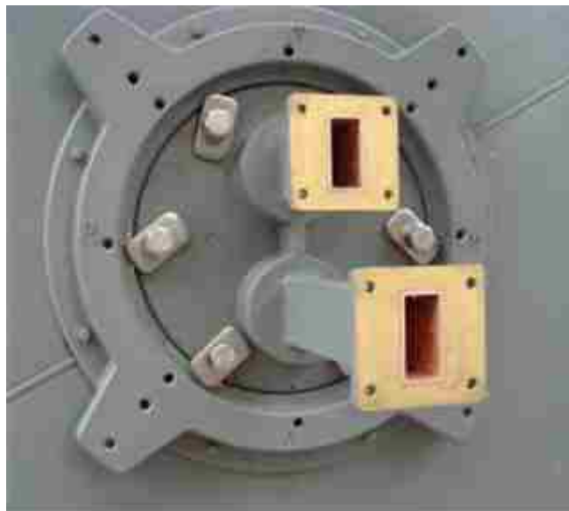
Figure 6-3 Feed boom of the separate-mount dual-polarized antenna
